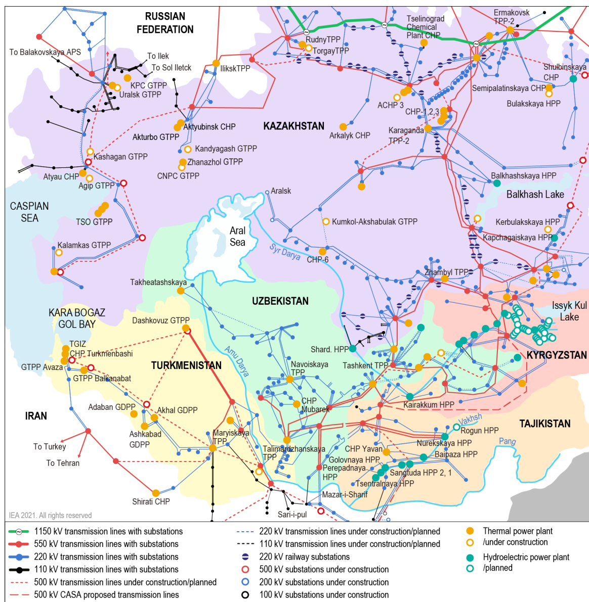
Figure 5 Central Asian power system, 2015
