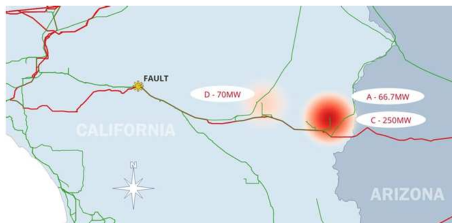
Figure 10. Western area outage of BESS caused by a misconfiguration and performance issue.
